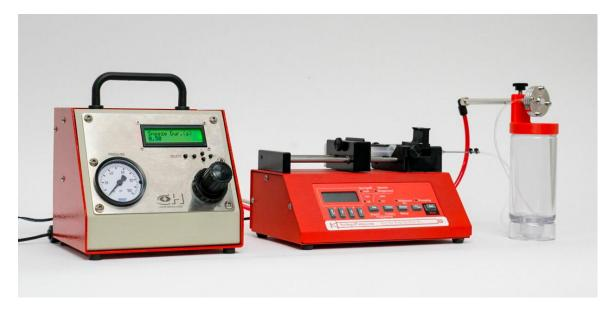
Figure 2: Syringe Fed Cough/Sneeze Mode
