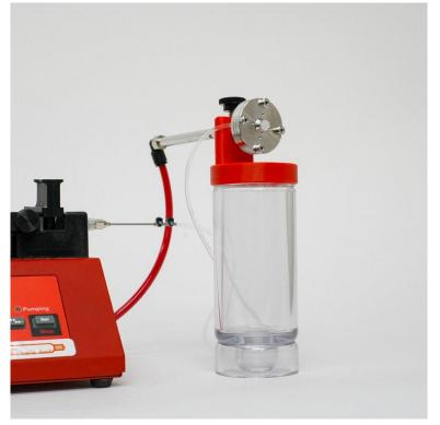
Figure 5: Syringe Fed Cough/Sneeze Mode Close Up
